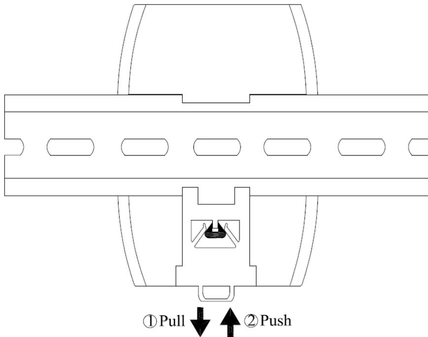
FIGURE 2: DIN-RAIL MOUNTING
