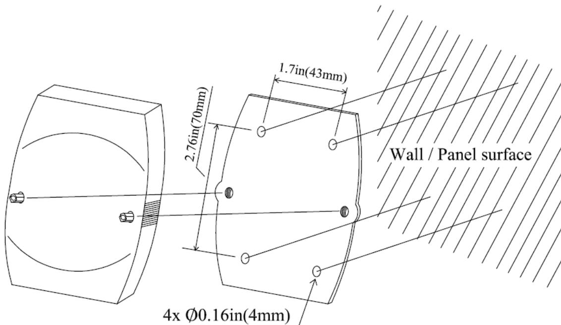
**FIGURE 3: WALL/PANEL MOUNTING**
