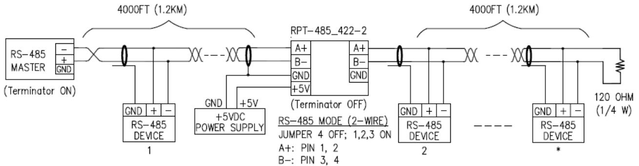
**FIGURE 1: TWO-WIRE RS-485 REPEATER**
