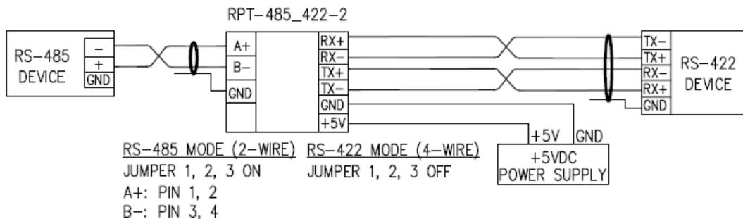
**FIGURE 3: TWO-WIRE RS-485 ⇔ FOUR-WIRE RS-422**
