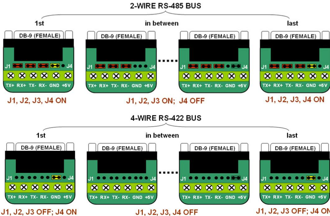
Turn on the 120Ω end-of-line terminator on both ends of the RS-485/RS-422 bus when the data rate is over 19.2kbps or the RS-485/RS-422's distance exceeds 660ft (200m).
