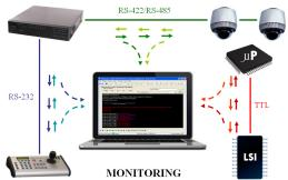
The 232Analyzer is capable of monitoring serial communications with direction indication and timestamps for long-hour recording. With the user-friendly logging window and options, reverse engineering has never been easier.
