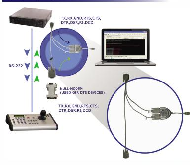
The 232Analyzer allows users to monitor full-duplex RS-232 communications with direction indication and timestamps. Not only is the data from both directions captured; the RS-232's signals (handshake line states) are also recorded in the logging window.
