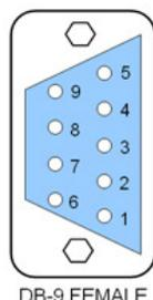
Note: Some software requires handshake line acknowledgements. To satisfy the requirements, the CVT-485-3's handshake lines (RS232 side) are tied together (DCD, DSR, and DTR tied together, CTS and RTS tied together). Therefore, you don't have to modify your existing software.
