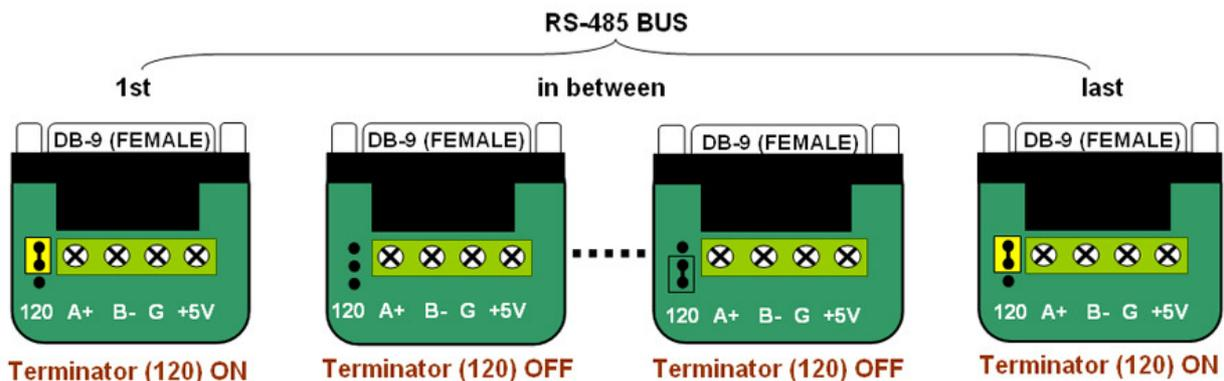
Turn on the 120Ω end-of-line terminator on both ends of the RS-485 bus when the data rate is over 19.2kbps or the RS-485's distance exceeds 660ft (200m).
