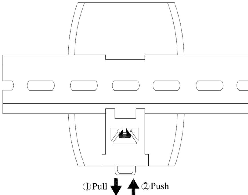
FIGURE 2: DIN-RAIL MOUNTING
