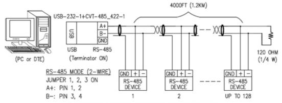
FIGURE 1: MASTER-SLAVE MULTI-DROP CONNECTIONS (RS-485)
