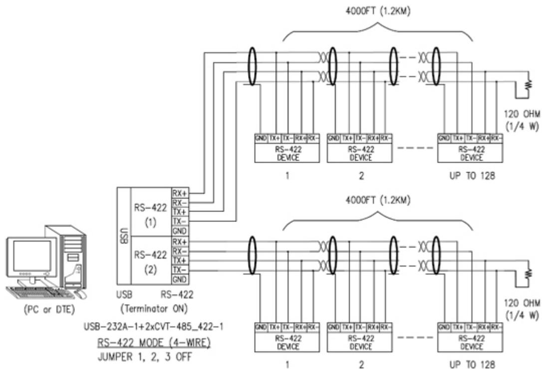
FIGURE 2: MASTER-SLAVE MULTI-DROP CONNECTIONS (RS-422)
