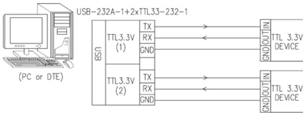
(FIGURE 1: USB-DUAL-TTL 3.3V CONVERTER CONNECTION DIAGRAM)
